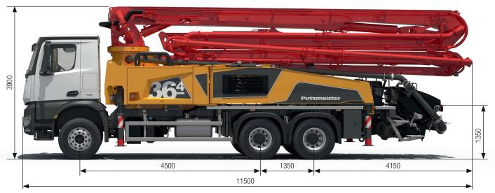
Note: Standard version. Dimensions and weights depend on truck, pump model and equipment. Dimensions in mm for MB-Actros 3243.
